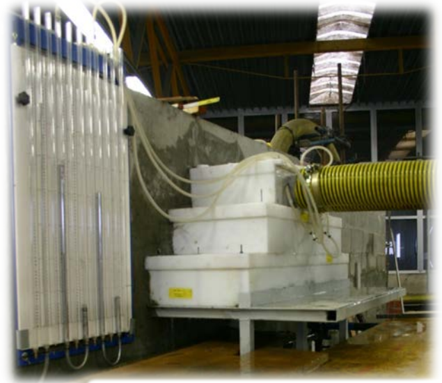
Fig. 7 – Physical model of the intake work (laboratory)
