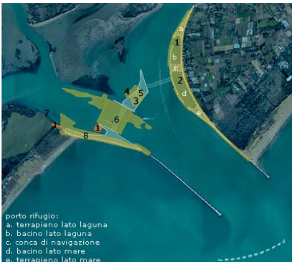
General layout of works underway and works finished at the Lido inlet
